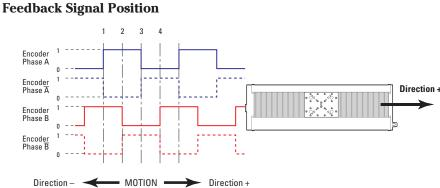
On FMS-CC stages, the incremental sensor operates following the photoelectric measurement principle, with a disk including slides.
